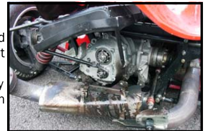
What’s wrong with this picture? Plenty as the hard impact shattered two gearbox covers, destroyed the rear wing, oil cooler, muffler and numerous other bits and pieces. Photo by L. Mason
